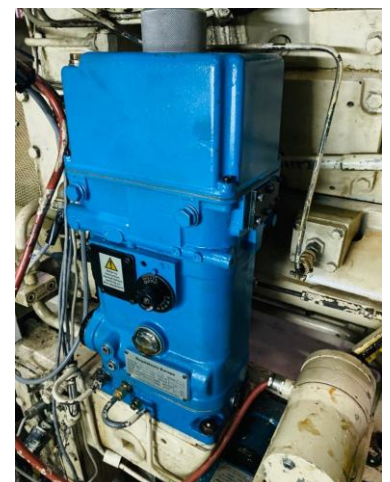
New Regulateurs Europa 1115 Model Installed on Engine
